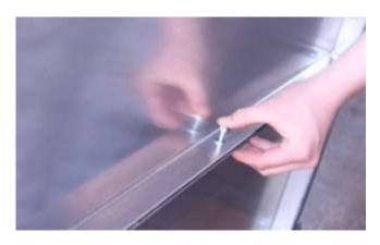
Mount the 4 screws per side to attach the lower side panels to the upper ones.
