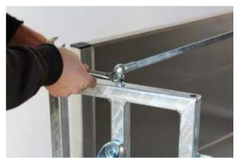
Fasten the rod and ball joint in the middle hole on the front door.
