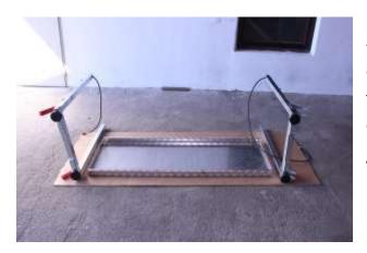
Lay the frame part with the wheel fastenings sideways on a flat surface. Be careful not to damage the attached cables.
