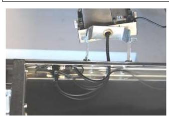
Thread the weighing signal cable of the indicator through the screw connection and down through the mounting bracket and connect it to the distributor. Attach the other two weighing signals to the distributor too.
