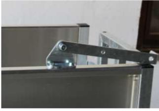
Attach the lever to the outside of the mounting bracket. The short part of the lever must face inward. The rounded head screw must point from inside to outside.
