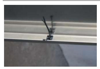
Thread one cable connector each through the latch of the self-adhesive cable brackets.
