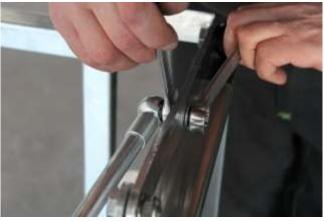
Fasten the rod with the second ball joint into the hole on the door lever.
